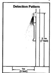
Once the B.Pir is installed and the cover replaced, the span and target direction of the detection pattern is set by gently turning the louver direction screws, located just below the detector lens on the barrel. As the adjustment range is about 45°, you must be careful not to turn the louvers too far; stop turning when resistance is felt. The slots on the louver adjusting screws indicate the position of the louver and serve as an adjustment guide. To adjust
