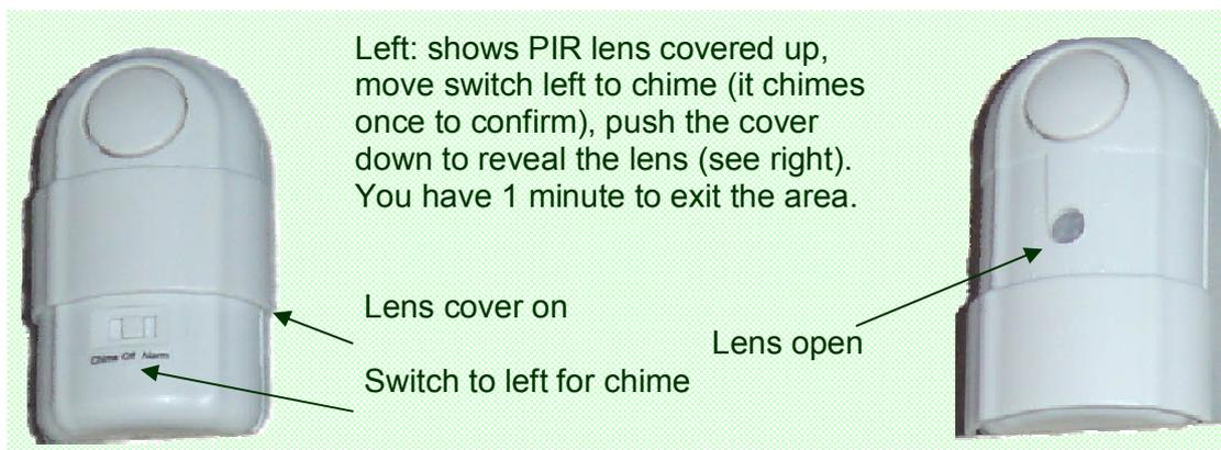
ChimeAlert™ has a field of detection of approximately plus/minus 20° and 4m max range. This narrow angle and short distance gives more flexibility in use. It enables set ups which would be impossible for a wider angle, longer range PIR
